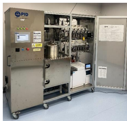
CO 2 Hydrogenation Reactor
