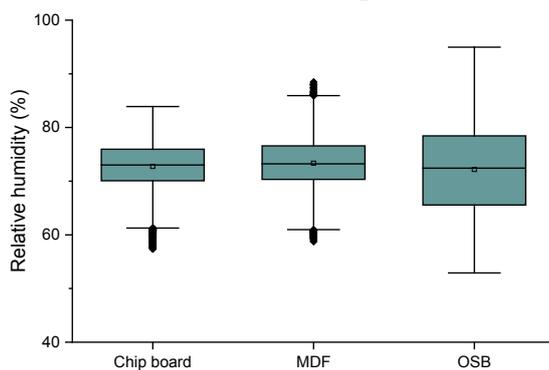
**Fig. 10** Effect of sheathing material on relative humidity in the interface between external sheathing and insulation
