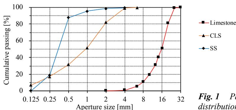
Fig. 1 Particle size distribution of aggregates
