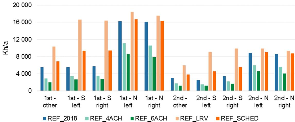
**Fig. 13** ODH<sub>26</sub> values in the reference building and with different ventilation/shading
