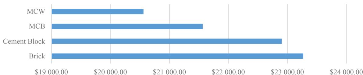
**Fig. 7** Life cycle cost of different walling materials (for 60 years) NPV as of 1st Jan 2017
