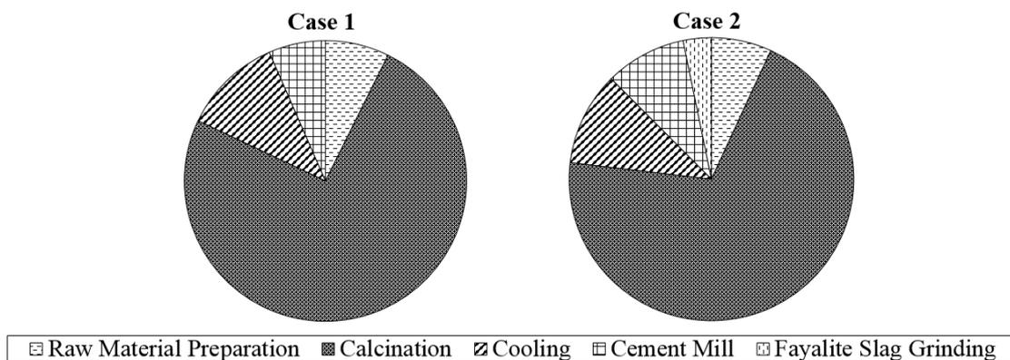
**Fig. 3** Exergy cost breakdown of the cement production (Note, the transportation cost for the SCM to the cement plant was not considered in this case study)
