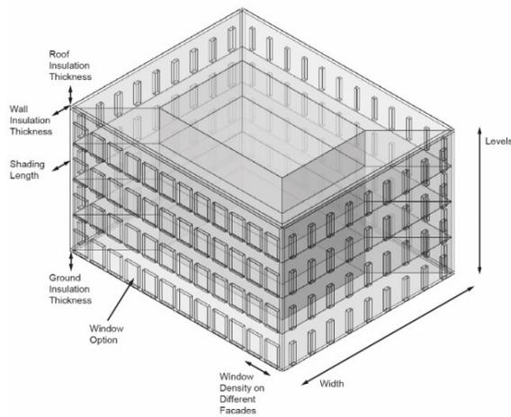
**Fig. 3** Thermal Zone model with Simulation Parameters presented
