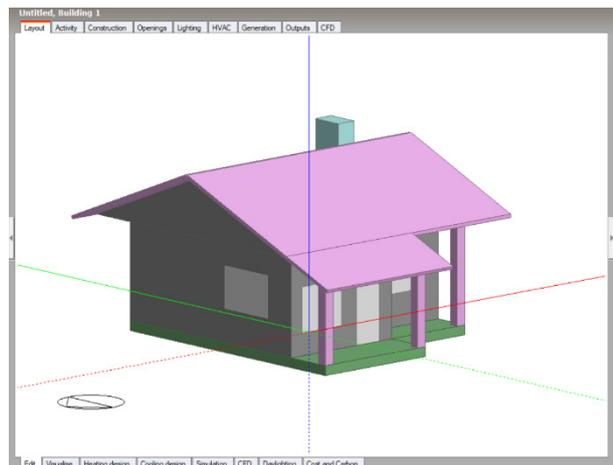
**Fig. 4** Modelled the basic house design on Design Builder software to calculate the cooling loads with different walling materials
