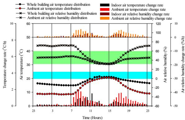
**Fig. 13** Average winter day whole building indoor weather condition response to ambient air temperature and relative humidity
