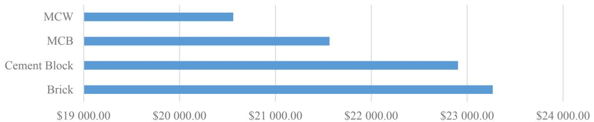
**Fig. 7** Life cycle cost of different walling materials (for 60 years) NPV as of 1st Jan 2017
