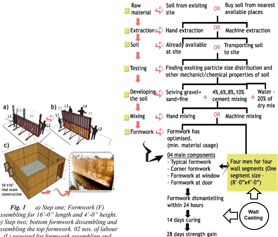
**Fig. 1** a) Step one; Formwork (F) assembling for 16'-0" length and 4'-0" height. b) Step two; bottom formwork dissembling and assembling the top formwork. 02 nos. of labour (L) required for formwork assembling and 02 labour (L) was required for mixing and pouring the MC mix.
