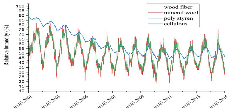
Fig. 7 Drying out process of structural element with different external insulations - wall type1
