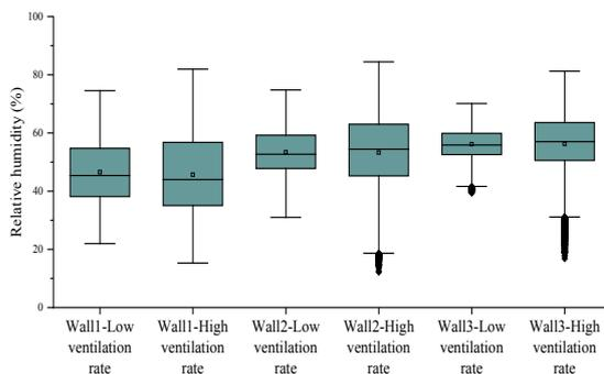
Fig. 12 Effect of ventilation rate in the air layer behind Façade on outer layer of structural elements
