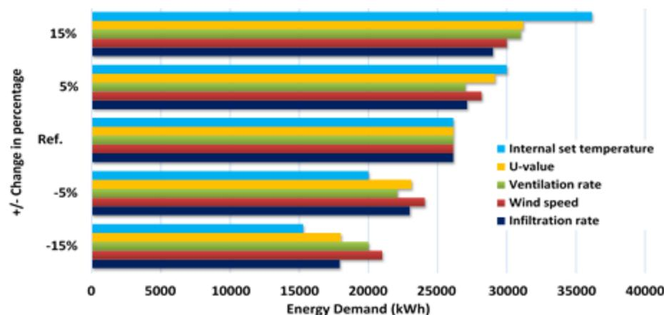
**Fig. 7** Local sensitivity analysis to investigate the influential parameter
