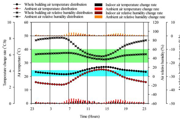
**Fig. 12** Average summer day whole building indoor weather condition response to ambient air temperature and relative humidity
