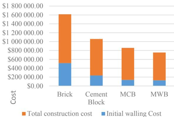
**Fig. 5** Total initial construction cost vs. walling cost
