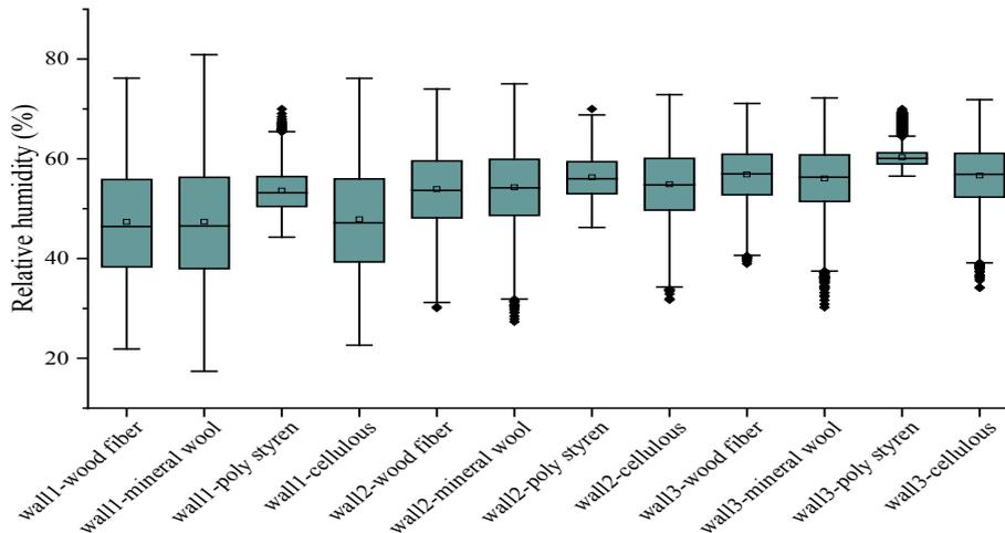
**Fig. 5** Relative humidity of the interface between external insulation and structural element – effect of different insulation materials
