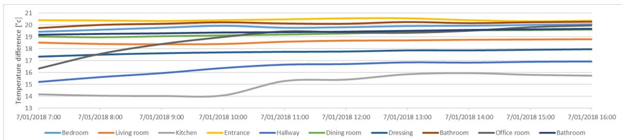
**Fig. 6** Air temperature per room, measured in dwelling 3 during a morning in the winter period.
