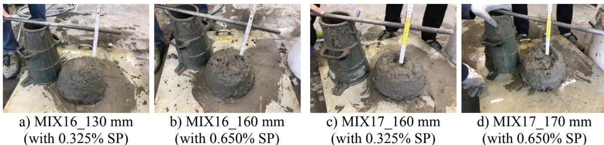
**Fig. 7** Workability of target mixtures
