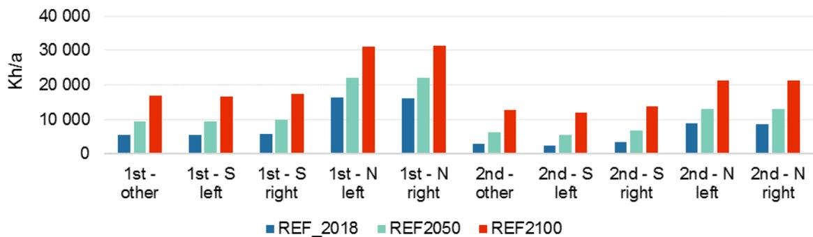
**Fig. 10** ODH<sub>26</sub> values in the zones of reference building according to 3 climate scenarios
