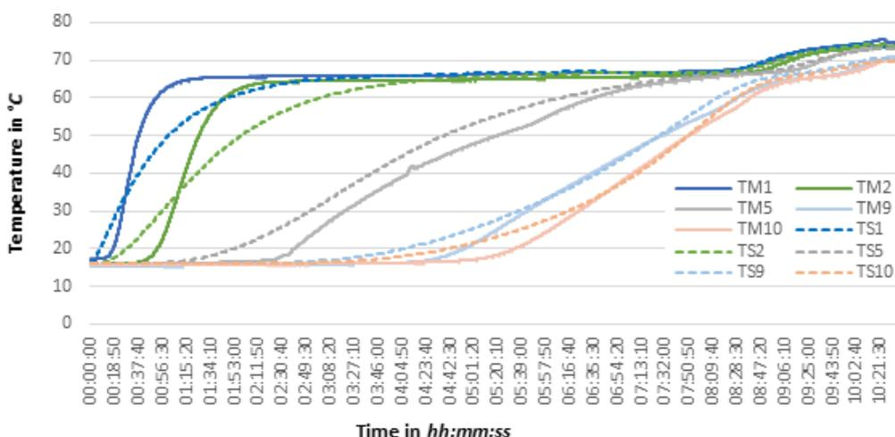
**Fig. 5** Comparison between measurements and simulations profiles for validation storage model
