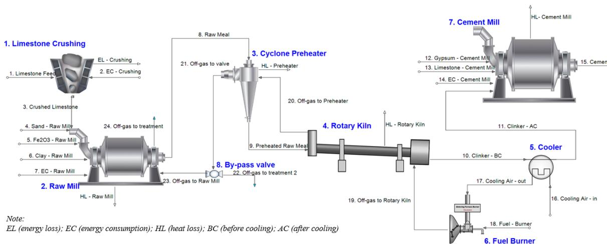
**Fig. 2** Flowsheet of the cement production process simulated with HSC Sim, showing the units considered and how they are connected between material and energy flows. This flowsheet would be linked to Fig. 1 to obtain a complete picture.
