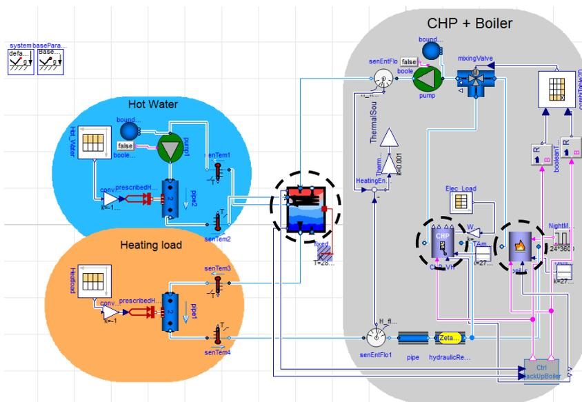
Fig. 2 CHP system Model Modelica.
