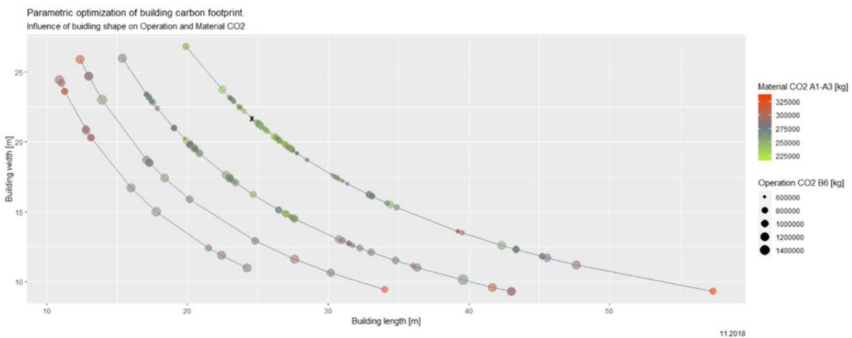
**Fig. 10** The effect of varying building dimensions on the Building Operation and Material related CO<sub>2</sub> emissions (the lines from the left to right represent Levels: 6 to 3 levels respectively; the “x” marks the optimal solution)
