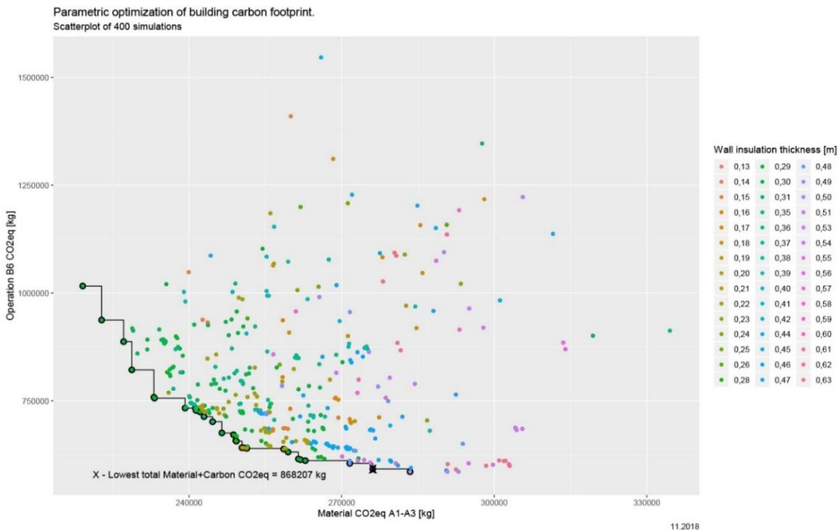
**Fig. 9** Scatterplot of all the simulations. Operation vs. Material CO<sub>2</sub>eq [kg]
