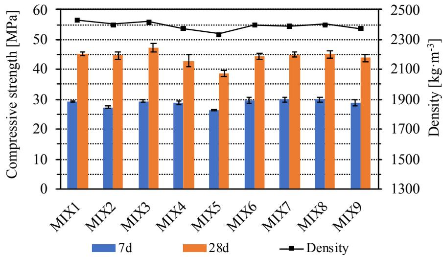
**Fig. 4** Compressive strength and density of MIX1 ~ MIX9
