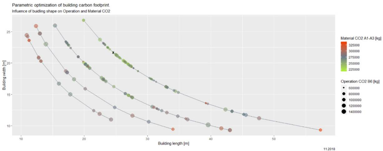
**Fig. 10** The effect of varying building dimensions on the Building Operation and Material related CO<sub>2</sub> emissions (the lines from the left to right represent Levels: 6 to 3 levels respectively; the “x” marks the optimal solution)
