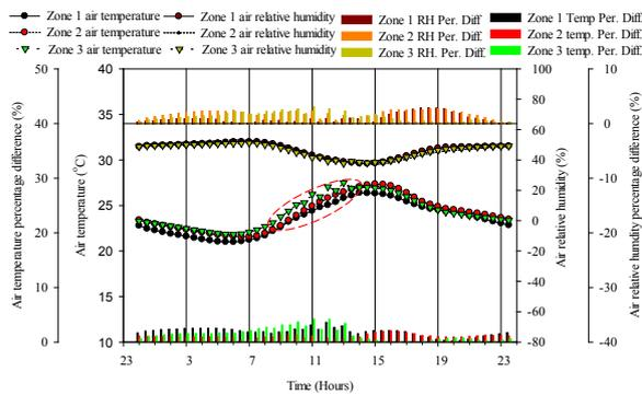
**Fig. 6** Typical summer day air temperature and relative humidity distribution in the various zones
