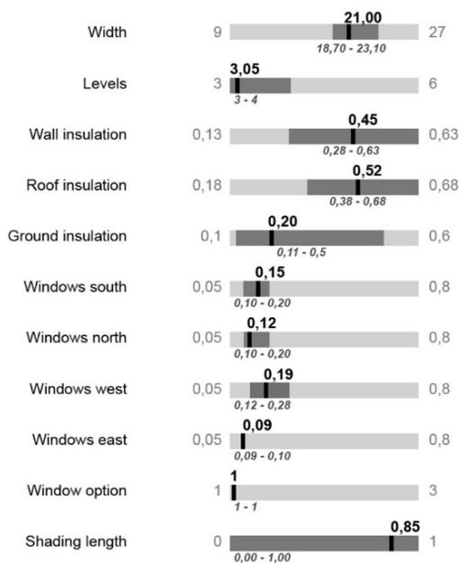
**Fig 11** The parameters of 20 best cases. Light grey shows the possible values. Dark grey shows the range of selections in the best 20 cases. The black tick represents the average value of the 20 best cases – "optimal" solution
