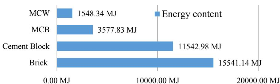
**Fig. 8** Energy content of building hundred square feet wall from different walling materials
