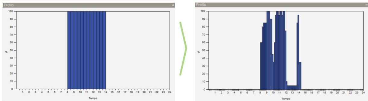
**Fig. 3** Behavioral profiles. On the left, traditional scheduling implemented into the simulation software. On the right, the behavioral profile due to the statistical analysis
