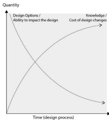
**Fig. 1** The design process – impact of the knowledge availability on the design options (based on [3],[11])
