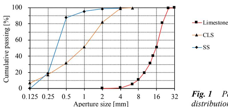
Fig. 1 Particle size distribution of aggregates
