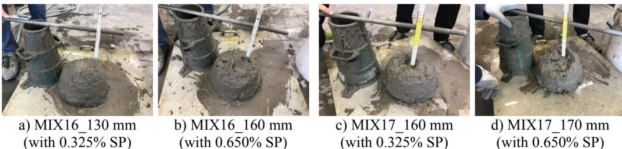
**Fig. 7** Workability of target mixtures
