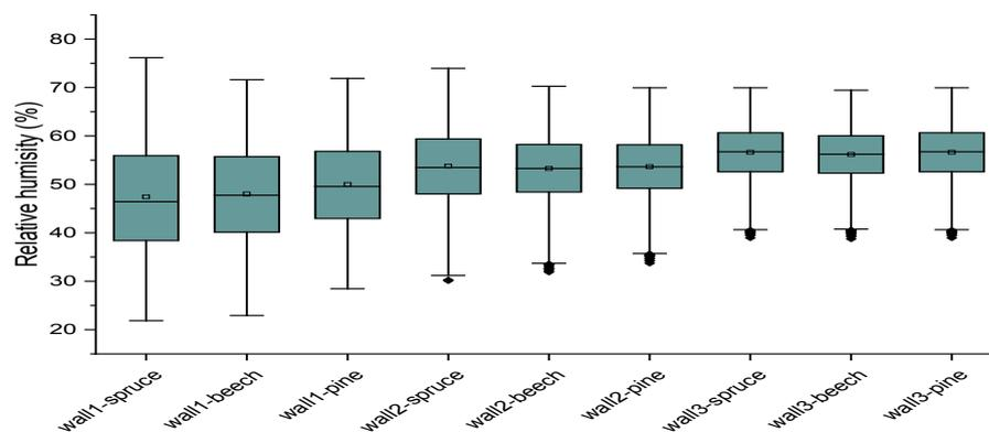
Fig. 8 Effect of different wood species on relative humidity of structural elements
