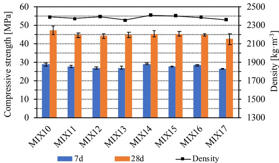
**Fig. 6** Compressive strength and density of MIX10 ~ MIX17
