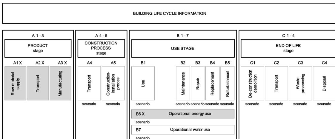
**Fig. 2** Building Life Cycle Phases, Phases marked with X (Grey background) have been considered in this study, (based on [10])
