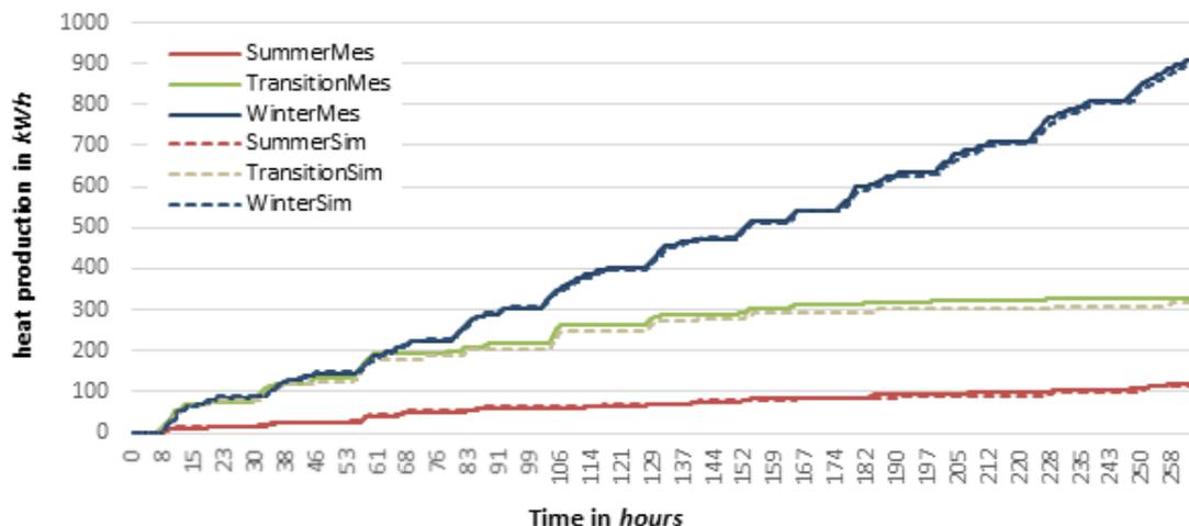
**Fig. 6** Cumulative heat production CHP-System
