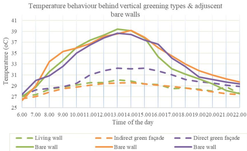
**Fig. 5** Temperature behavior of wall surfaces shaded by vertical greening compared to adjacent bare wall controls
