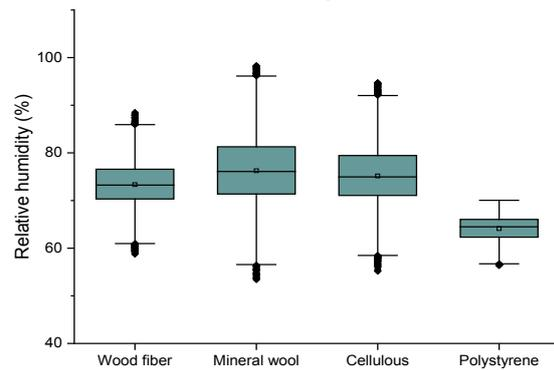
**Fig. 11** Effect of insulation material on relative humidity in the interface between external sheathing and insulation
