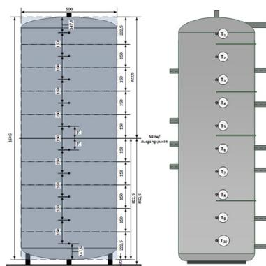
**Fig. 4** Measuring points and layers.
