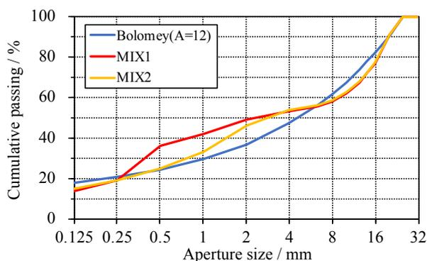
**Fig. 3** Optimization through the Bolomey's grading curve
