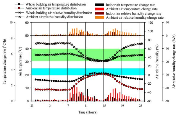
**Fig. 13** Average winter day whole building indoor weather condition response to ambient air temperature and relative humidity
