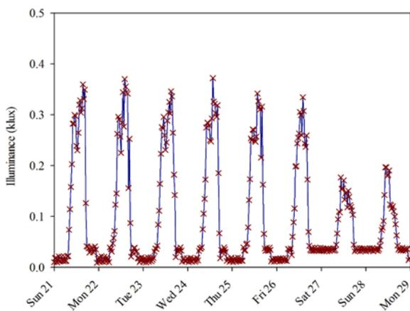
**Fig. 14** The passive solar house indoor illuminance distribution
