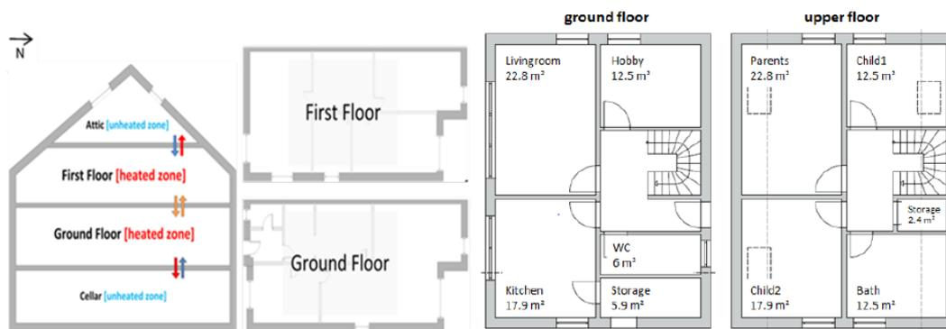
Fig. 1 A schematic drawing & floor plan of the selected One Family Dwelling in Aixlib.
