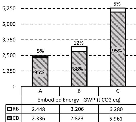
**Fig. 1** Embodied Energy results (Construction and five years maintenance)
