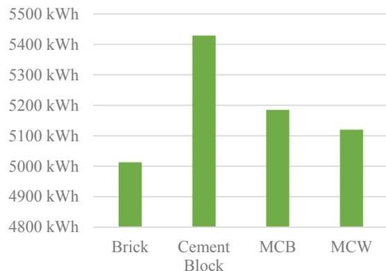
**Fig. 6** Cooling load calculation for 60 year
