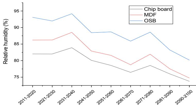
**Fig. 9** Maximum Relative humidity of each decade in the interface between external sheathing of panel and internal insulation layer - with different sheathing material – wall type 3
