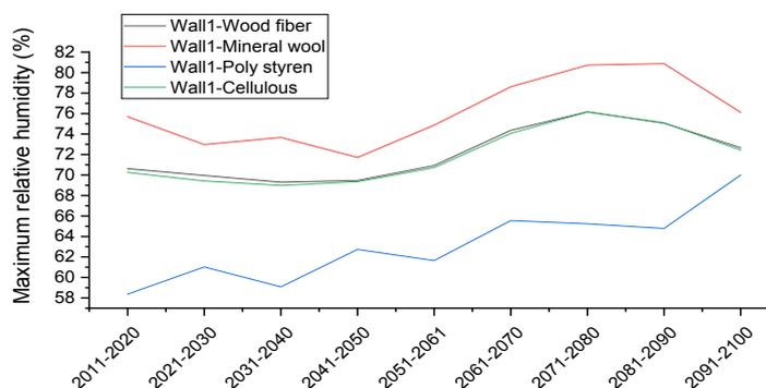
**Fig. 6** Maximum Relative humidity in each decade in the interface between external insulation and structural element – effect of different insulation material
