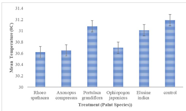
**Fig. 8** Mean temperature of the wall surfaces shaded by the green panels
