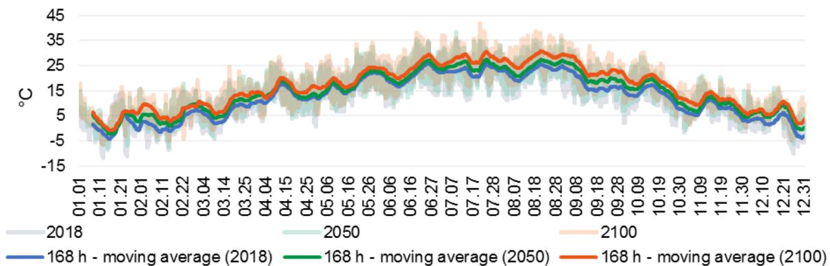
*Fig. 8 Temperature values according to the 3 scenarios*
