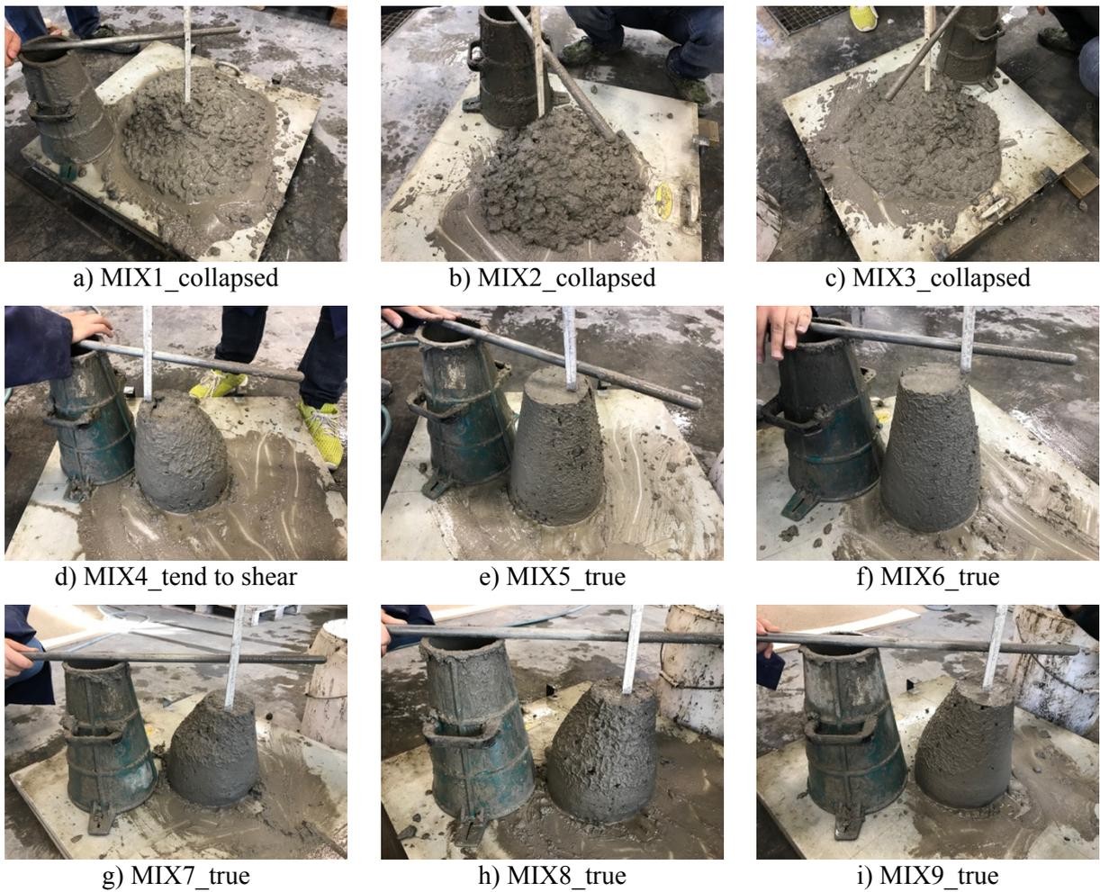
**Fig. 5** Photographs of slump test of MIX1 ~ MIX9
