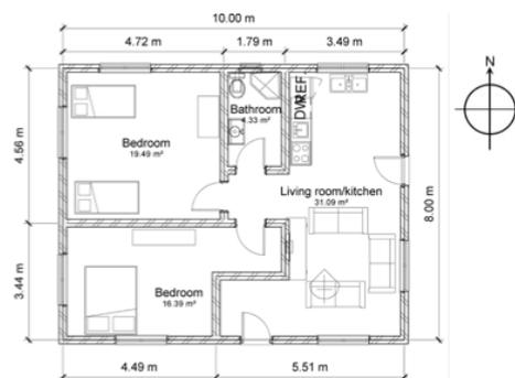
**Fig. 2** Space layout of the passive solar house
