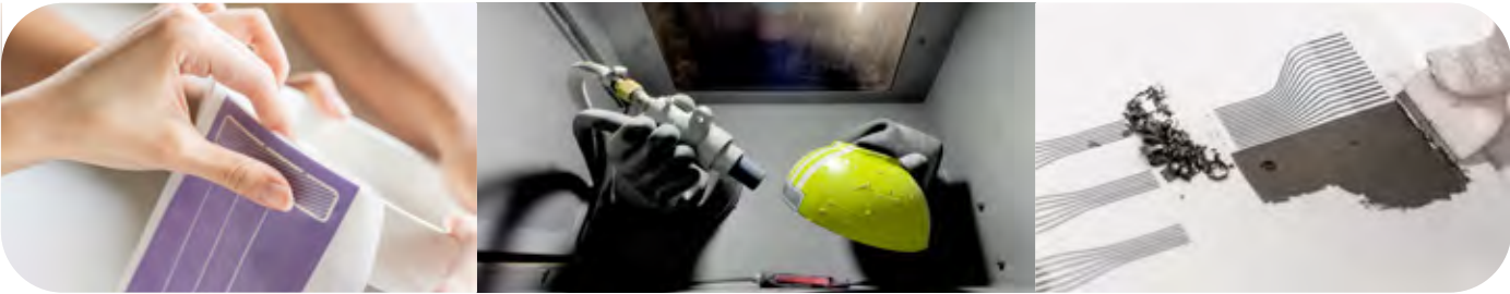
(From left to right) Applying the vinyl mask onto a glazed ceramic object, sandblasting a masked ceramic object, scraping excess conductive ink away to reveal the functional circuit underneath
