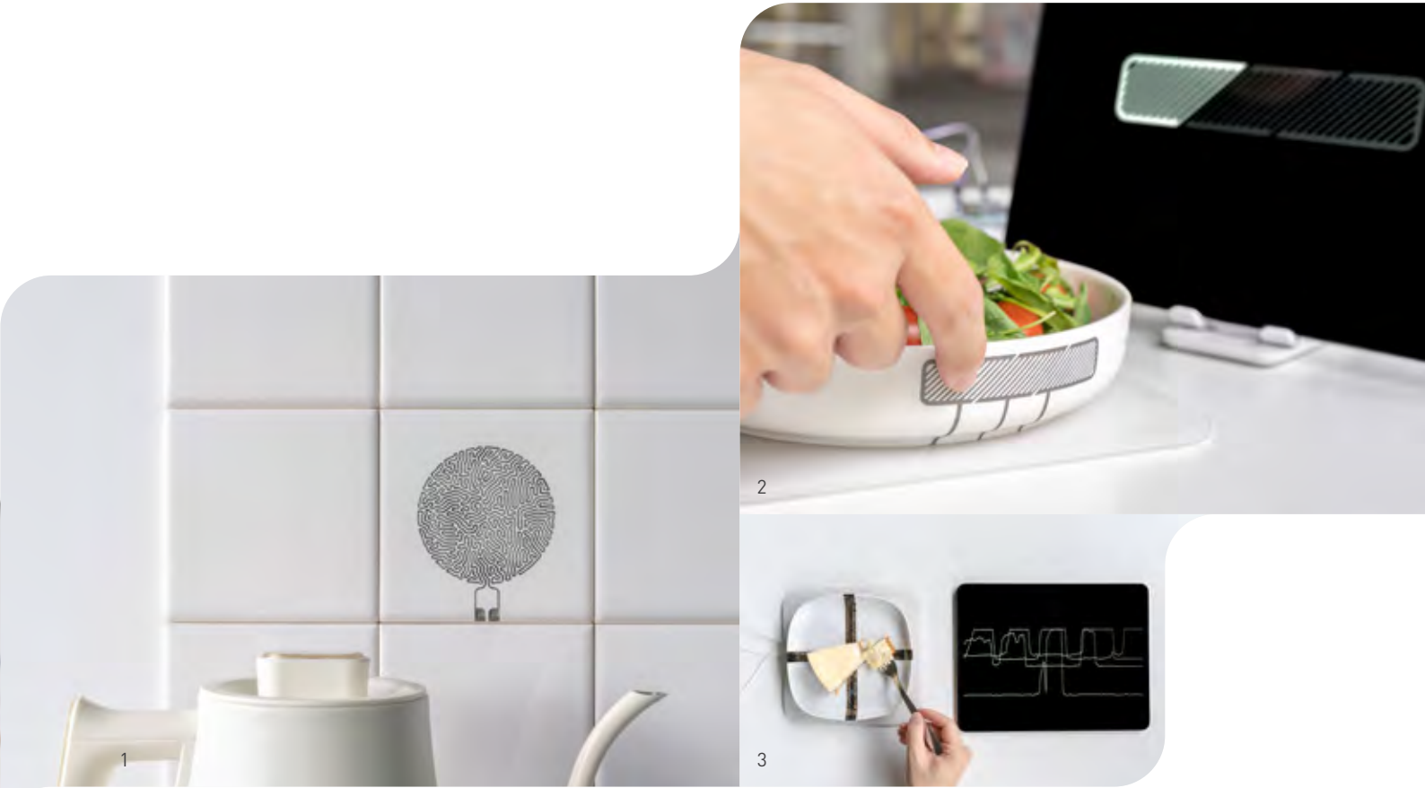
(From 1-3) Temperature sensing kitchen tile, salad bowl with touch slider, dessert plate for tracking eating activity
