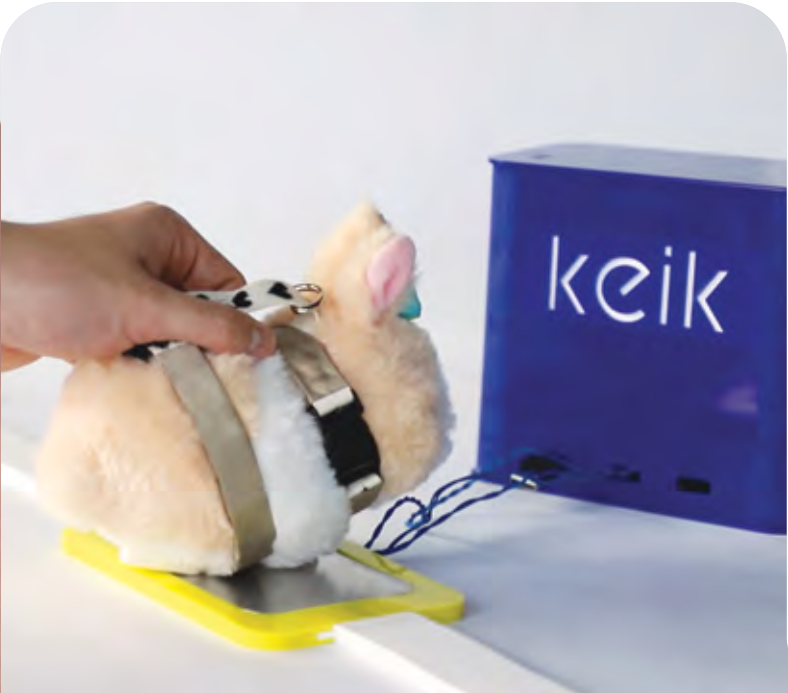
Keik Keik is the collision of physical and digital play. It uses a harness to 'power up' existing toys in the house to be played in a digital gamescape. This balances the stimulation of the digital screens with the imagination of physical play. It utilises different metals to differentiate multiple inputs.
