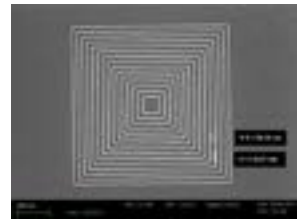
Nested structure with Pitch 20 nm & linewidth 5 nm
