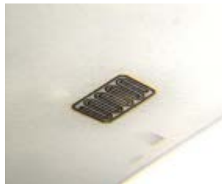
Laser micro-machining of macro features on Silicon Nitride and Ceramic material
