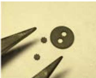
Laser micro-machining of macro features on Silicon Nitride and Ceramic material
