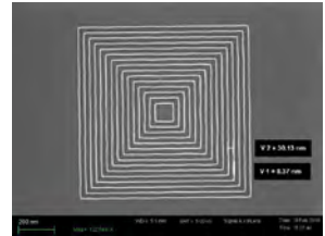
Nested structure with Pitch 20 nm & linewidth 5 nm
