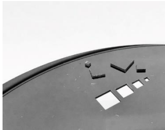
Precision Laser micromachining of Si wafer.
