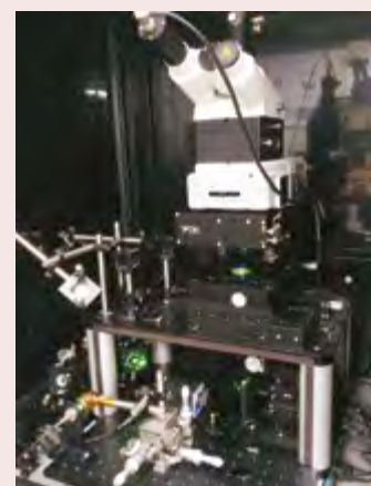
Figure 2: The confocal microscope where the nanosieve [Figure 1(b)] is placed and illuminated by green light. It is used to observe the hologram in Figure 1(b).
