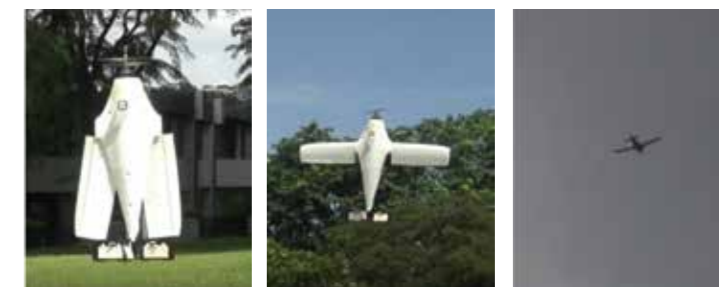
Wings closed while hovering Wings open while hovering Cruise flight
