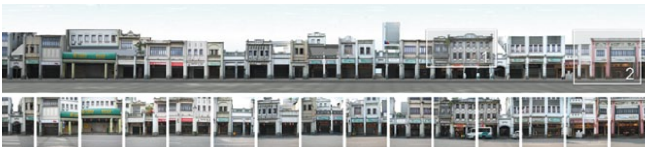
Figure 2: An example result of the ‘image-based facade modelling’ system: some input images in the bottom row, the recovered model rendered in the middle row, and three zoomed sections of the recovered model rendered in the top row
