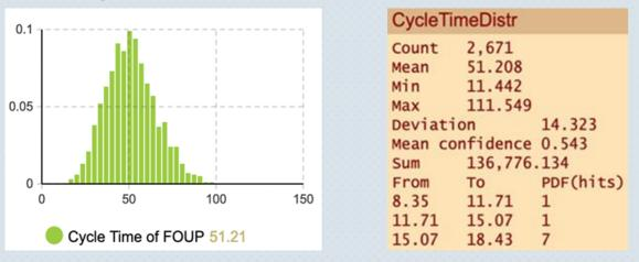
Average FOUP waiting time: Measures the time from when the vehicle is activated to time the vehicle arrives to load the FOUP.
