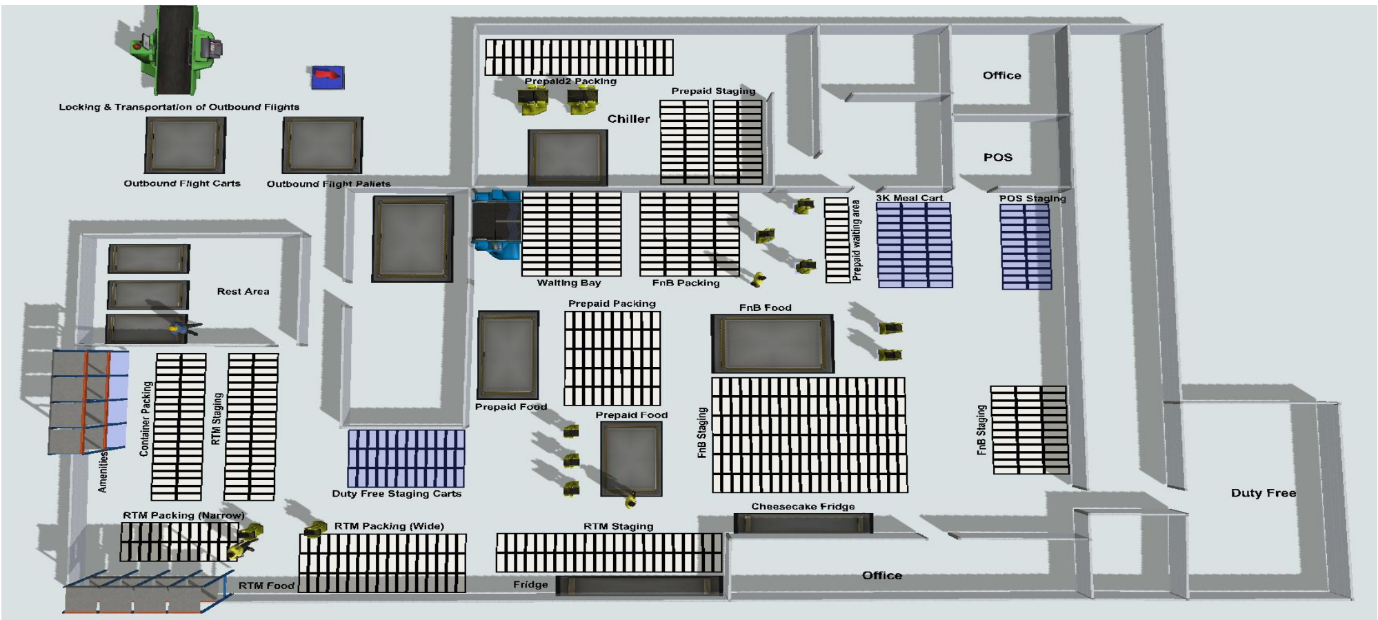
FlexSim 3D model that simulates the operations and workflow of packers
