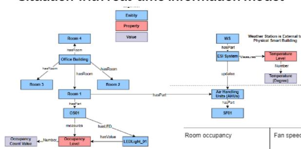
Same process flow as without real-time information model, but include the collection of real-time data on outside temperature and occupancy at 30-minute intervals
