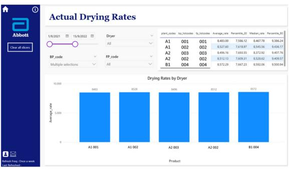
The default view for the PowerBI dashboard has sliders to filter data by date and drop down lists for filtering by dryer or BP/FP code. The selected data is then displayed in the given table and as bar charts.
