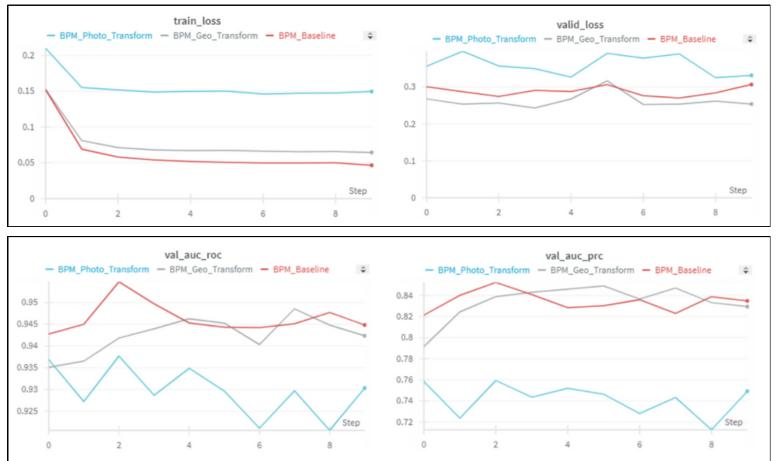
The baseline binary classification model has the lowest training and validation loss. AUC ROC value is also the most favorable for the baseline binary classification model, and the baseline model is also the best performing model based on comparison of
