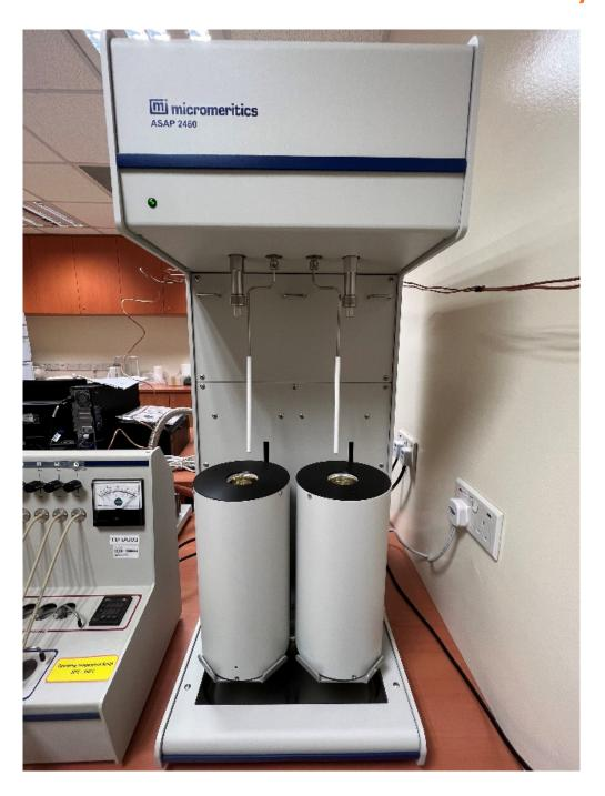
The ASAP 2460 is a high-performance adsorption analyzer for measuring surface area, pore size, and pore volume of powders and porous materials. The ASAP 2460 is ideally suited for gas adsorption analysis of mesoporous (2 to 50nm) materials and delivers superior accuracy.
