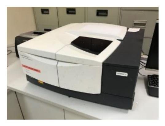
FTIR spectrometer is used for measuring how samples transmit, absorb, scatter, or reflect EM radiation in the IR (Infra-Red) range, typically in mid-IR.
