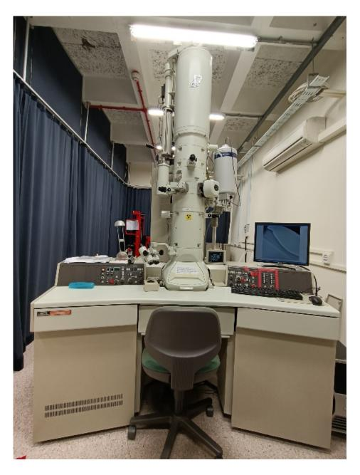
The JEM-3010 Electron Microscope, a 300KV ultrahigh resolution analytical TEM (transmission electron microscope), has been born out of the ultrahigh resolution, micro-area analysis, electron diffraction, and convergent beam electron diffraction techniques.
