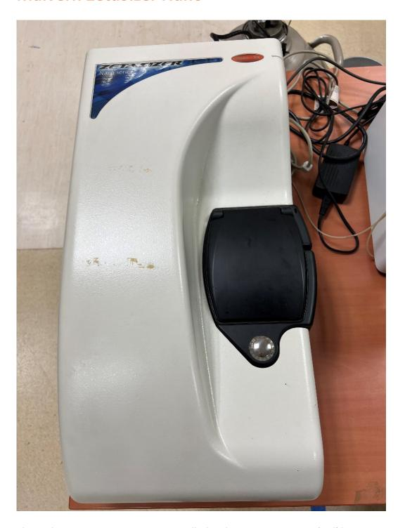
The Malvern Zetasizer Nano ZS is installed with a 4 mW 632.8 nm 'red' laser. It is able to test Particle size range: 0.6nm - 6 $\mu$ m. Size range for Zeta potential: 5nm - 10 $\mu$ m.
