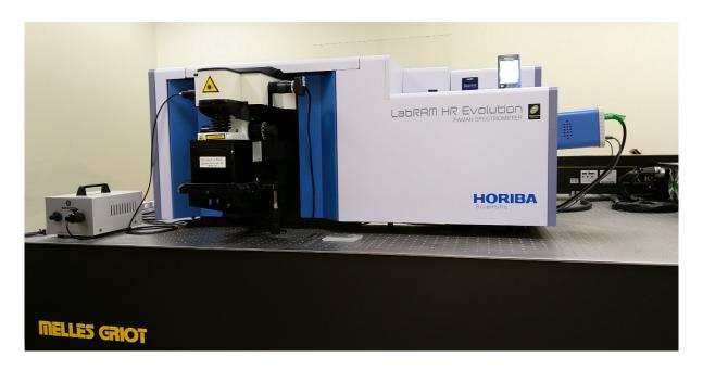
Raman spectroscopy is a light scattering technique used to determine vibrational modes of molecules and can provide detailed information about chemical structure, phase and polymorphy, crystallinity and molecular interactions.
