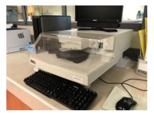
The step profiler is an instrument for measuring the thickness of a film or the depth of an etch on a flat sample.
