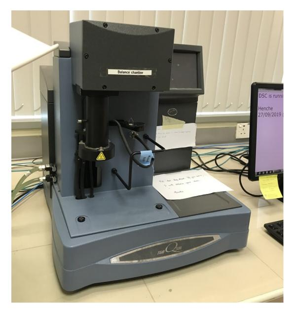
The TGA is an instrument for measuring mass change of a sample when it is heated. It can be used for determining, for example, the mass loss due to thermal decomposition as well as the onset temperature of the decomposition.
