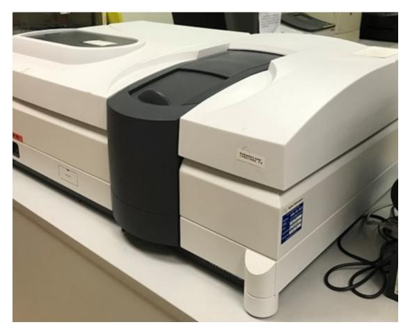
Our unit can be used for transmittance or absorbance measurements of liquid samples or flat thin film samples, and also the specular reflectance of thin flat film samples with mirror-like surface.
