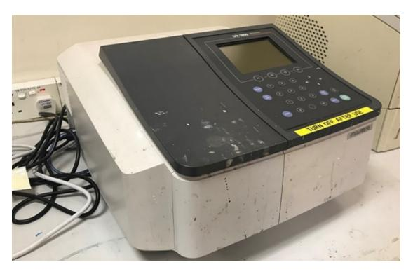
UV-Vis spectrometer is an instrument used for measuring how samples transmit, absorb, scatter, or reflect EM (electromagnetic) radiation in the ultraviolet range and visible light range of the EM spectrum.
