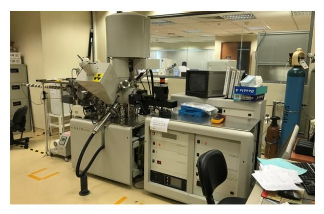
XPS system is an instrument for analyzing the photoelectron emission peaks from the surface of samples, which provide information about what element are present, their relative quantity, and their chemical states.
