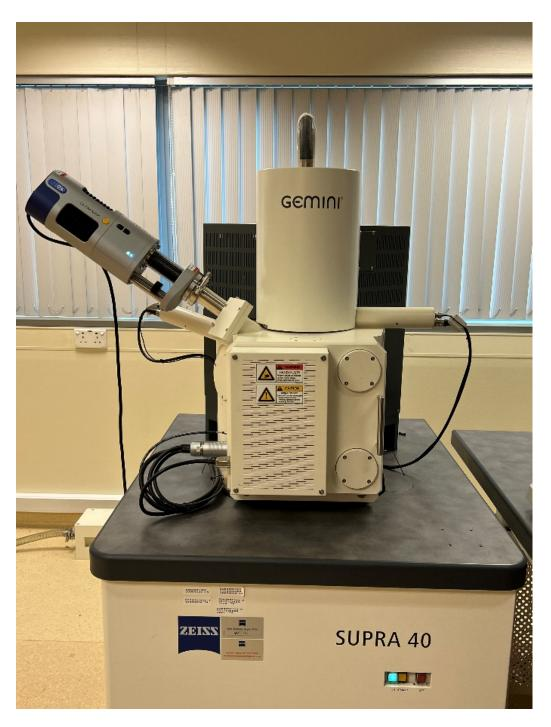
The Zeiss Supra 40 FE SEM is the Schottky field emission (SFE) source provides excellent beam brightness, unsurpassed probe current stability and probe current suitable for quantitative analytical applications.
