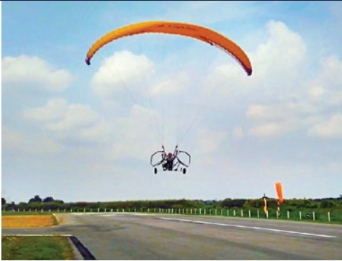
The Delta weighs just 49 kg, and can fly up to a speed of 36 km per hour under normal wind conditions, for a typical flight time of 10 minutes on fully charged batteries.
